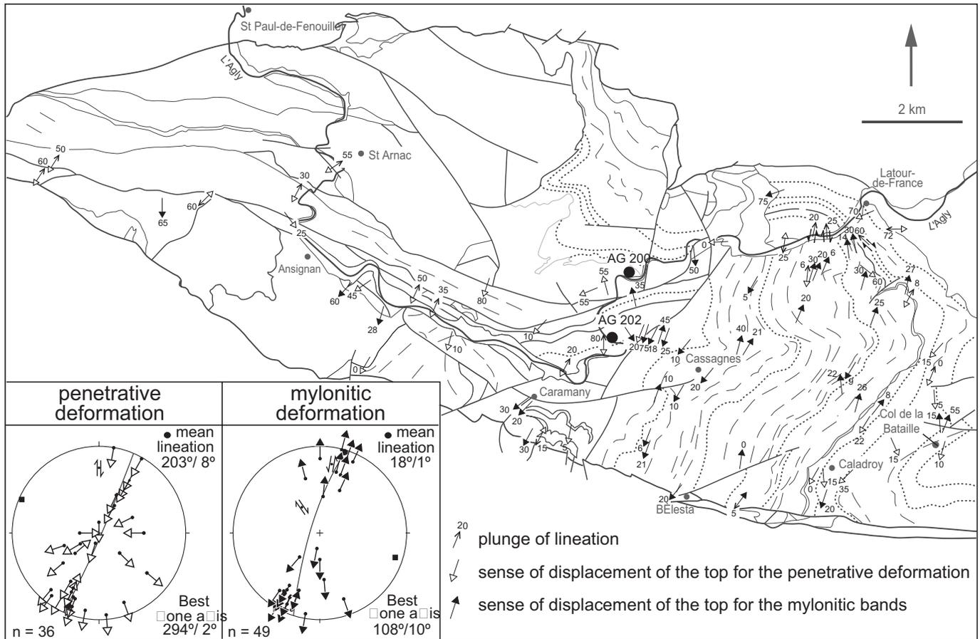
Figure 4. Map of the lineations corresponding to unambiguous senses of shear, for the pervasive and the mylonitic deformations, determined on XZ thin sections. Stereonet (Schmidt, lower hemisphere, 1% area contours) of the foliation poles and of the lineation for both deformations. AG 200 and AG 202: location of the deformed granites dated in this paper.
