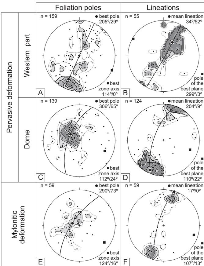
Figure 3. Stereonets (Schmidt, lower hemisphere, 1% area contours). (A) Poles of the major pervasive foliation and its associated stretching lineation for all the Agly Massif. (B) Poles of the mylonitic foliation and its associated stretching lineation for all the Agly Massif.
